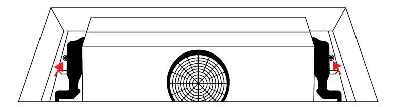
Obstructions can be removed either by compressed air or nitrogen, or physically removing the obstruction with a drain cleaner. DO NOT use a chemical drain cleaner, as this will void the warranty and possibly damage the unit.
