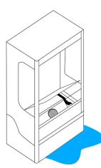
The drain lines can be accessed by removing the bottom panel from inside the unit.
