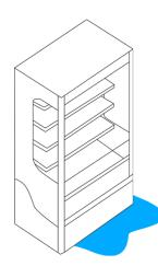
Over time it is likely that the drain lines will become clogged which will result in water overflowing the condensate pan and onto the floor. This is a standard maintenance item and will not be covered under warranty.
